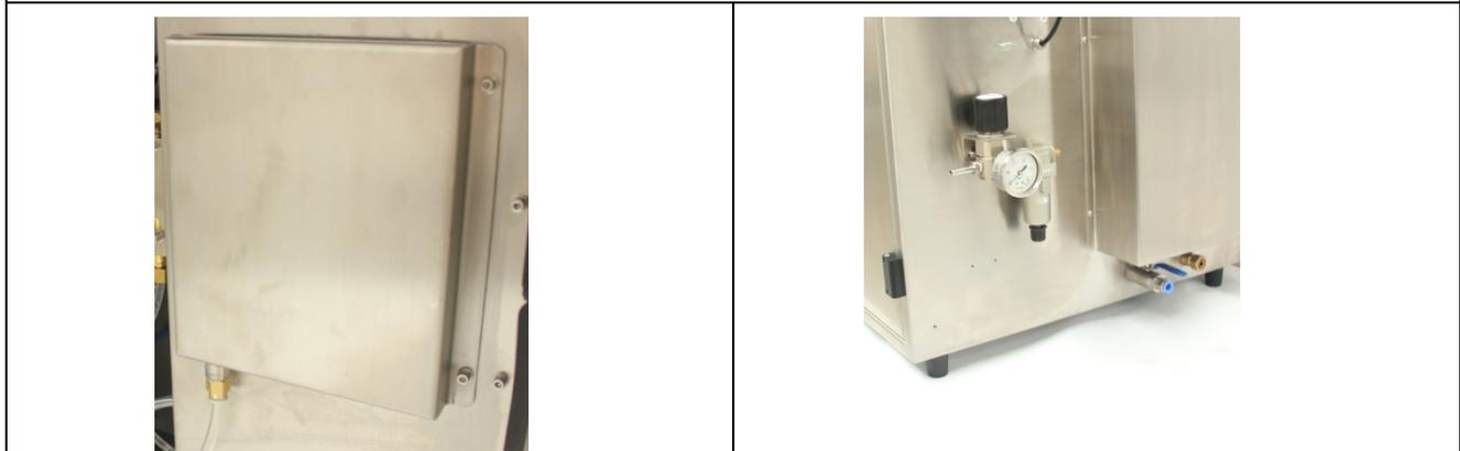
Water collecting box is installed on the side door of test station and labyrinth water eliminator is installed inside the collector to develop the ability of releasing pressure when the bottle burst. Release the pressure in time and reduce water splitting from the top of the door.
