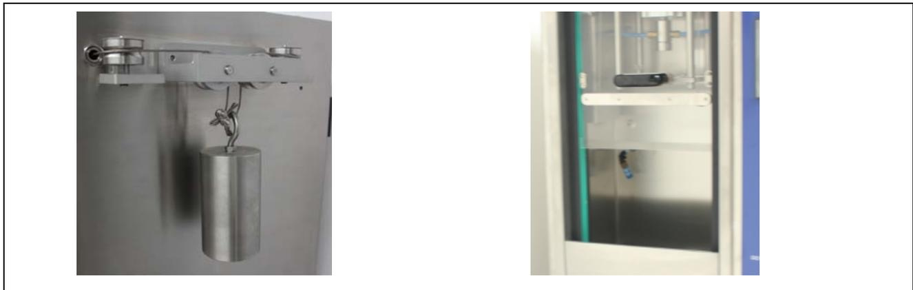
Weight hammer is assembled for lifting or pulling down the door, saving effort of operators and preventing injury causing by door falling down. Improved friendly operation.
