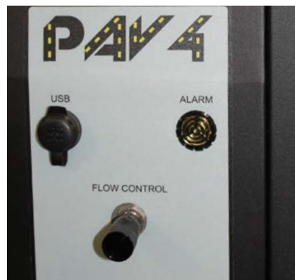
Figure D.4: Flow Control valve
