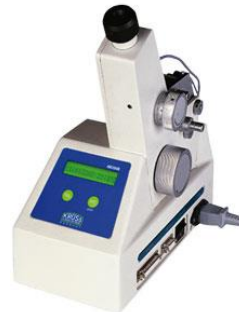
AR2008 Series Abbe Refractometer
