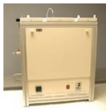
Oxidation Stability Tester (RPVOT/RBOT), ASTM D2112, D2272
