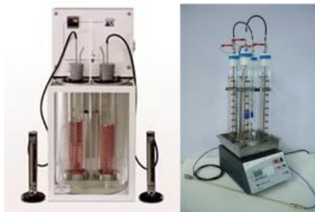
Foaming Tester, ASTM D892+Diffuser Washer
