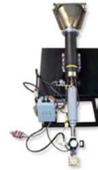
FAA Oil Burner (NexGen) Insulation Flame Penetration
