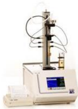
Automated Cold Filter Plugging Point (CFPP), ASTM D6371
