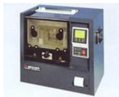
Dielectric Breakdown, ASTM D877
