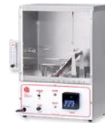
45° Flammability (Apparel Textiles)
