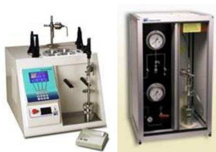
OXIDATION STABILITY OF GASOLINES - AUTOMATED , ASTM D525
