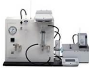
Air Release Value Tester, ASTM D3427
