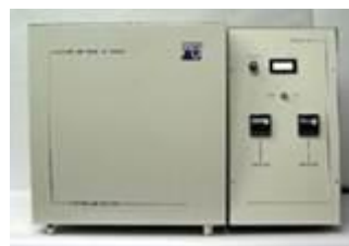
EXISTENT GUM IN FUELS BY JET EVAPORATION, ASTM D381
